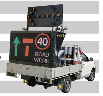
For Trucks & Utes: Fixed or Flush mounted, Colour LED display
